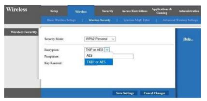
After choosing the encryption mode, the device will allow you to set a Pre-Shared Key (PSK) (better known as a WPA2-PSK), which is used during the authentication phase between the wireless router/access and the client. The WPA2 security mode uses a 256-bit key for data encryption of all traffic to and from the client.
